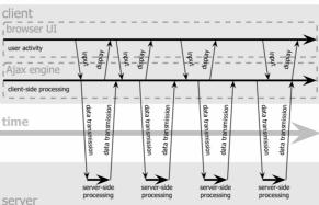
Figure 5: The synchronous interaction of traditional Web application (top) compared to the asynchronous pattern of an Ajax application [9].
