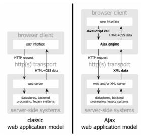
Figure 6: Traditional model of Web application (left) compared with the Ajax model (right) [9].
